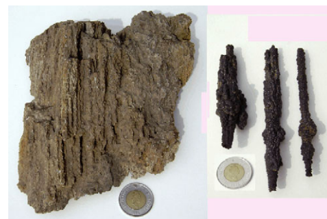
Pipe ore (left) from the Pennington iron ore bank located west of Pennsylvania Furnace, PA, and (right) iron ore speleothem from Connecticut (see text). Coins are 1.1 inch across. R. Altamura photos
