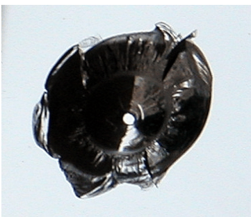
Hertzian cone fracture in glass, photo by user Polyparadigm, 2005, used under CCA-SA 3 license
