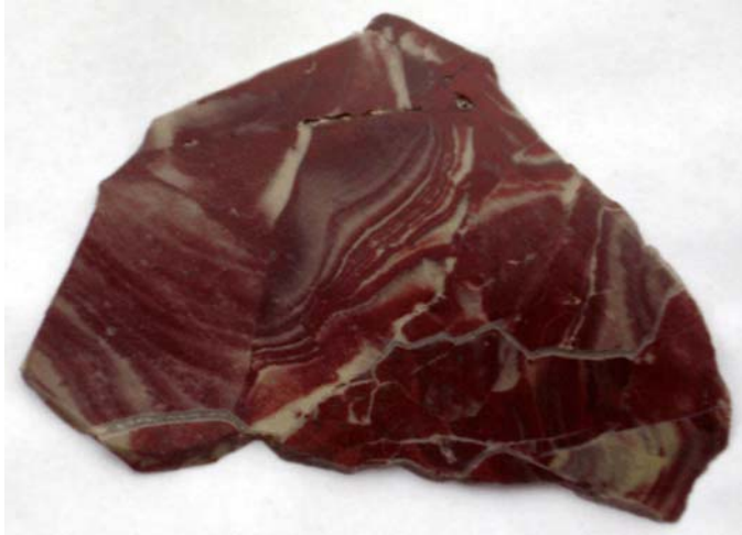
A sawn slab of red banded jasper, 4.9" It is thoroughly lithified, should behave well if carved. R. Altamura photo.
