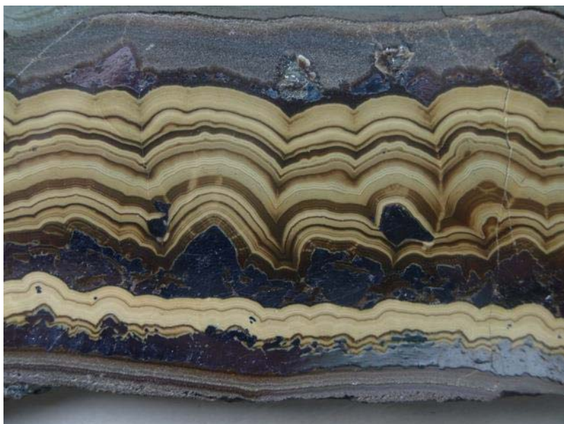
Schalenblende, Olkusz District, Poland. This 2-inch-high slab of schalenblende probably consists of layers of galena (bottom), sphalerite and wurtzite, and marcasite (top). The marcasite formed last and is slowly disintegrating. Photo: Tom Tucker.
