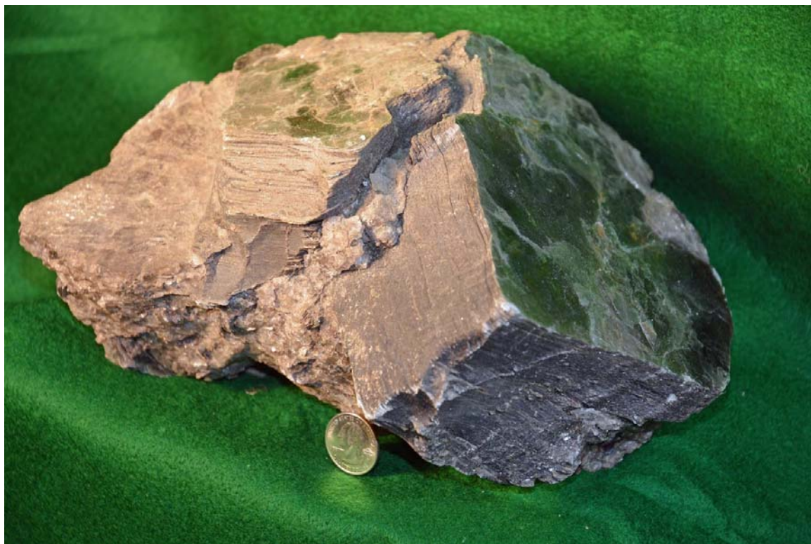
Figure 1: Pegmatite specimen (measuring 11" x 7.5" x 5") showing a 2.6-inch-thick book of muscovite mica (right half of image). Delaware, 1973. Basal cleavage of the mica is well shown. Collected and photographed by the author. Note quarter for scale.
