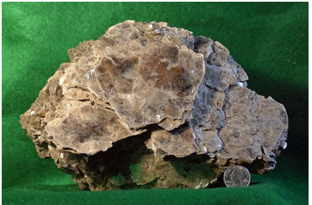
Figure 3: Hand specimen of muscovite mica (10" x 4.5" x 5.5"); Delaware, 1973. Note quarter for scale. Collected and photographed by the author.
