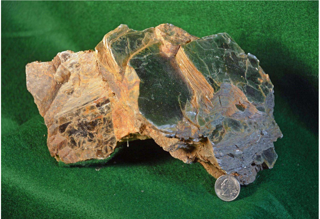
Figure 2: Pegmatite specimen (9" x 6" x 5") with 3-inch-thick book of muscovite mica. Other minerals include quartz and feldspar. Delaware, 1973. Note quarter for scale. Collected and photographed by the author.
