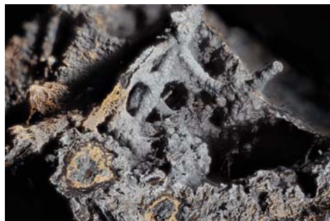
Goethite (based on color and brown streak) rod forms in a vug in freshly broken lump ore from the Scotia pit. Minor tan minerals appear to be alteration products. Field of view approx. 1 inch across. J. Passaneau photo
