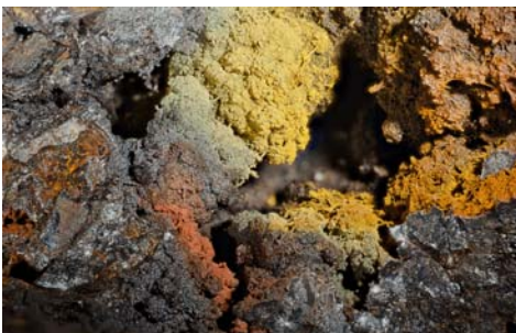
Limonite and goethite in a vug in freshly broken lump ore from the Scotia pit. Field of view approx. 1 inch across. J. Passaneau photo
