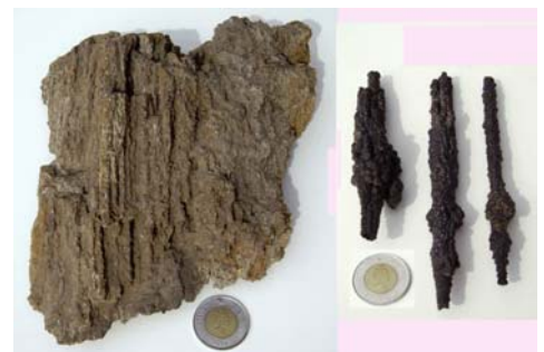
Pipe ore (left) from the Pennington iron ore bank located west of Pennsylvania Furnace, PA, and (right) iron ore speleothem from Connecticut (see text). Coins are 1.1 inch across. R. Altamura photos
