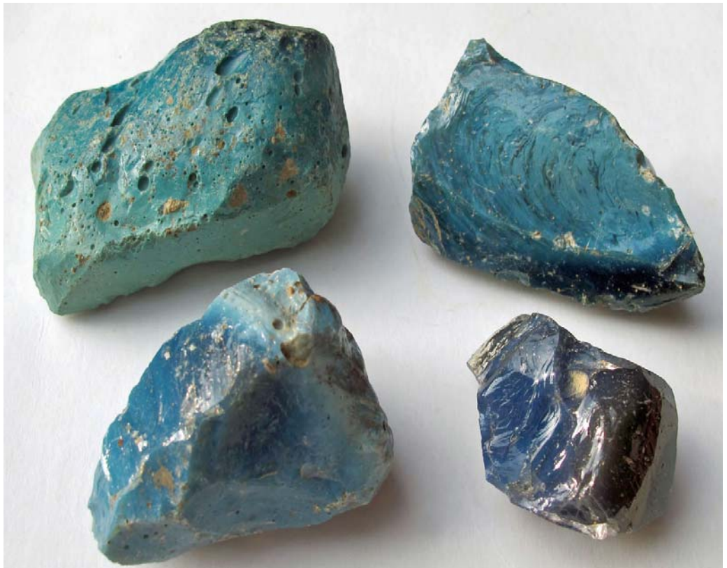
Iron furnace slag from central Pennsylvania, found by Jim Garthe. Note the gas bubbles in the specimen at top left, swirls of color at top right, and conchoidal fracture at bottom right. D. Glick photo
