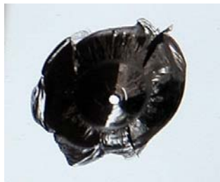
Hertzian cone fracture in glass, photo by user Polyparadigm, 2005, used under CCA-SA 3 license
